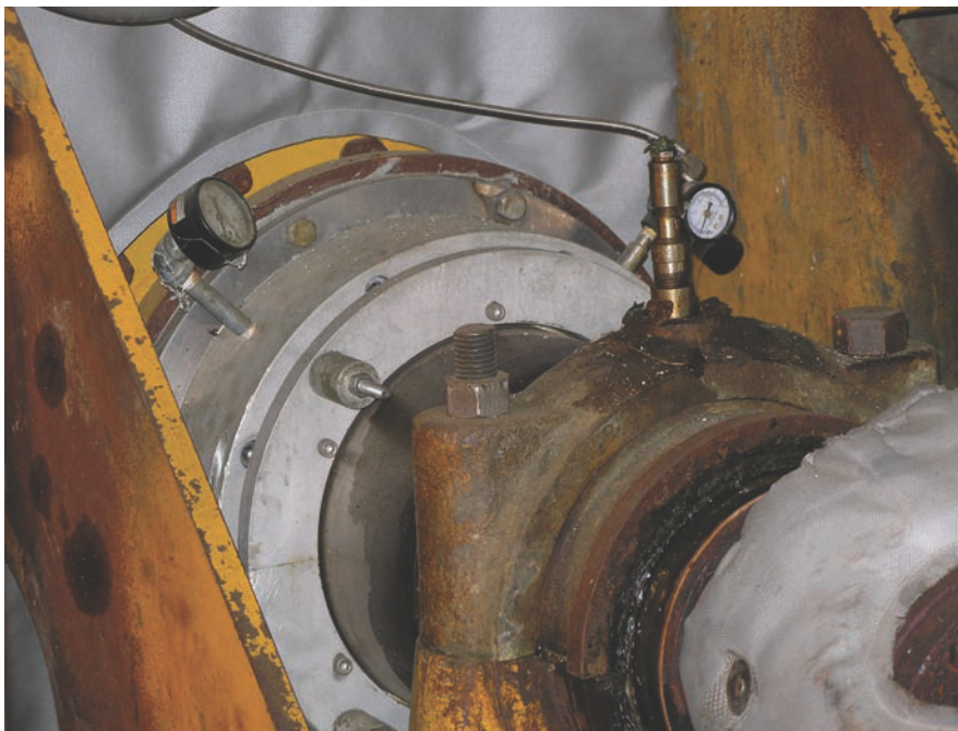
A pressure gauge monitors the seal purge pressure, keeping it at least 2 psi above the dryer's pressure in order to ensure and maintain a perfect seal.
