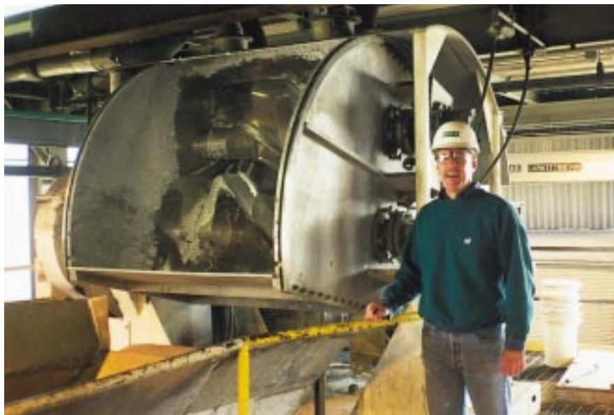
Michael Keslin, production manager at W.R. Grace, can now wear normal work clothes when operating the plant's sigma blade mixer.
