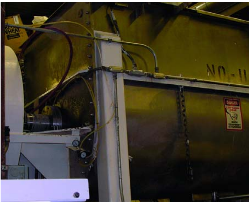
Blender 11 is a 4,000-pound-capacity ribbon blender that mixes up to 12 batches of specialty blends per day with the new shaft seals installed.
