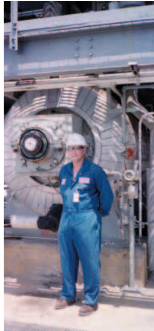
DuPont's mechanical engineer Chris Marshall improved the performance of this vacuum dryer by installing MECO shaft seals on it.
